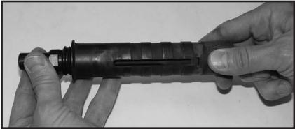
UNSCREW THE MUZZLE BUSHING FROM THE BARREL
