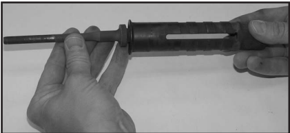
REMOVE PISTON OUT OF THE BARREL
