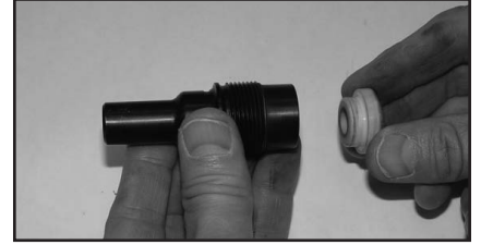
PULL THE BUFFER OUT OF THE MUZZLE BUSHING
