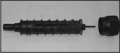
SLIDE THE BARREL ASSEMBLY AND BARREL SPRING OUT OF THE TOOL BODY
