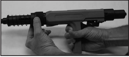
UNSCREW THE BARREL RETAINING COLLAR
