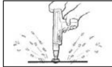
NEVER FASTEN INTO VERY HARD OR BRITTLE MATERIALS
